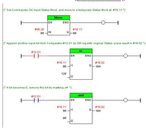
In this manner, a Fieldbus host can read and decode the new I/O Status Word placed and #18.02 in our example program above, and pick up our new added bit in the bit 7 position.
