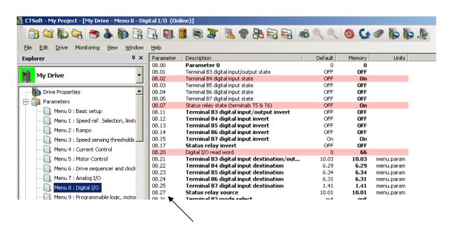
It should be noted that in this example we could have cheated..... if the relay on T5/T6 were not being used for anything, we could simply set #8.27 = 12.01 and the I/O Status word would then reflect the state of #12.01 within bit 6 of the original #8.20 word. But then we wouldn't need a SyPT Lite program to accomplish this - this would have certainly simplified this Application Note example.
